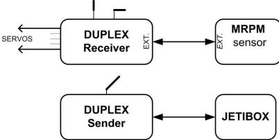
**3.** Connect the three-wire cable with JR connector to the Jeti Duplex Expander module and ensure that the Expander module is connected to the Duplex receiver. In this configuration the sensor is powered through the expander, which is powered through the receiver. Switching on the transmitter and receiver allows the sensor to be configured appropriately for your power system and alarm settings to be defined.
