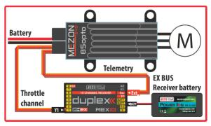
**Pic. 2**-standard connection between controller and receiver suitable for JETI Duplex transmitters users
