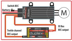
**Pic.1** - standard connection between controller and receiver suitable for **JETI Duplex** transmitters users
