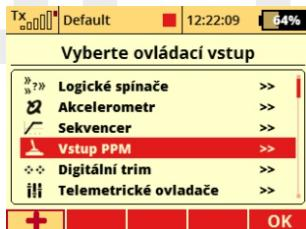
**EN** - You can find the assignment of the switch connected via the MSW expansion module in the menu of PPM input (see figure).
