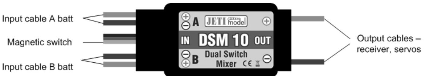
Be sure to correctly connect the input and output cables, red cables must always be connected to positive poles, black cables to negative poles.
