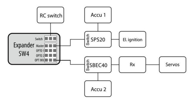
Fig. 1: Expander SW4 application connection
