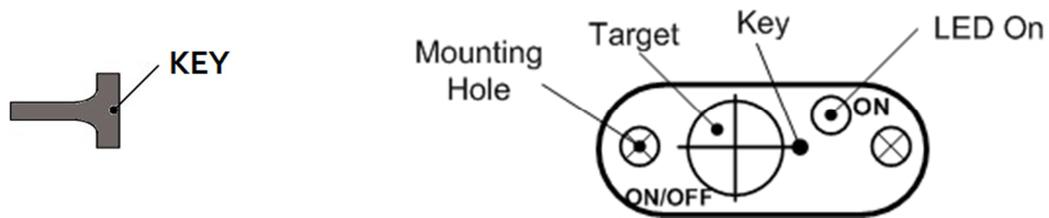
When you correctly position and hold the magnet on the target as described, after 1 sec the green LED will turn on as a steady light, showing that the electronic switch is ON. Switching off is done in a similar way. When the magnet touches the target in the proper orientation again and is held in place for 1 sec., the green LED turns off and the system switches OFF.
