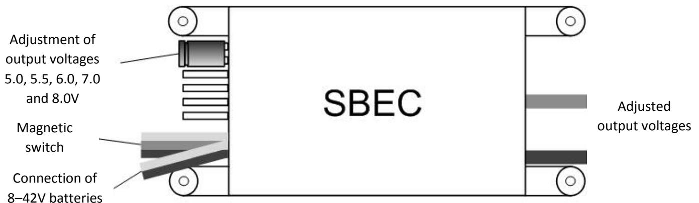
Wiring diagram of the regulator:
