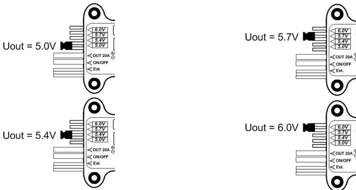
Using the JETIBOX terminal, navigate to the *Output (x.x) Volt* setting (See section “*SETTING - Configuration Options*”) and change to your desired value. This can be done in steps of 0.1V independently of the position of the short-circuit/jumper plug.
