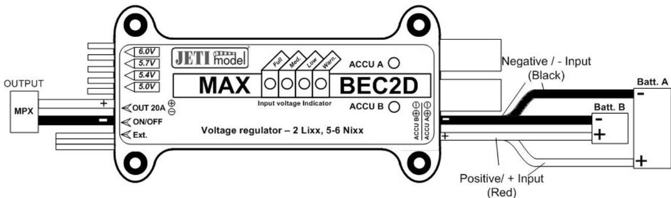
To connect your device(s) to the MAXBEC2D PLUS, either solder your wires (Please use wire of at least 1mm<sup>2</sup> diameter or larger, depending on your anticipated load) to the MPX output connector of the MAXBEC2D PLUS or use the JETI MPX/3xJR cable, available separately. The Duplex EPC receivers, such as the R6 EPC, R8 EPC, R12, R14 and R18 are already fitted with a compatible MPX plug.
